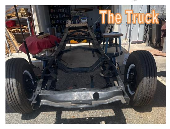
Update on truck finished chassis 90% bolts replaced new brakes front and back wheel cylinder /kingpins / all wheel bearing/ front shocks/universal joints 3 center bearing on tail shaft just have to do plumbing for back brakes. Need Front ball for steering next job is to fit motor and gearbox make hand brake and fit tail shaft then touch up paint .
