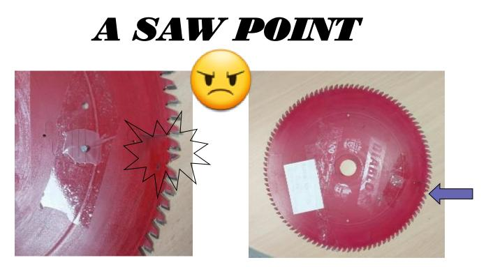
Somebody put some timber which contained a steel nail through the saw recently damaging the blade (see pictures). Due to the damage the blade has to be replaced at a cost to the shed of \$150—\$190. Please remember chaps that it is mandatory to scan your timber with the scanner before putting it through the saw. The scanner is located between the two drop saws. If you aren't sure how to operate the scanner please ask someone how to.
