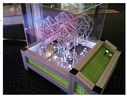
After all the parts were cut out the edges were scratch-polished to remove the machine marks and the bearings glued-in (all 228). Dowel pins made and the walking machine assembled.
